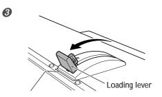
Pull back the loading lever to secure the media in place.
