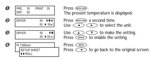
By default, simply switching on the power does not make the machine warm up to the preset temperature. Pressing (SET UP) to make the light come on makes the system warm up to the preset temperature.
