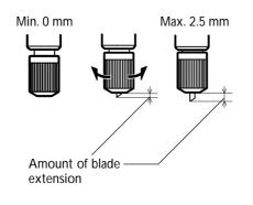
When you want to perform accurate and fine adjustment of the cutting-in amount, such as when cutting media with thin carrier paper, you can obtain good results by adjusting the tip of the blade.
