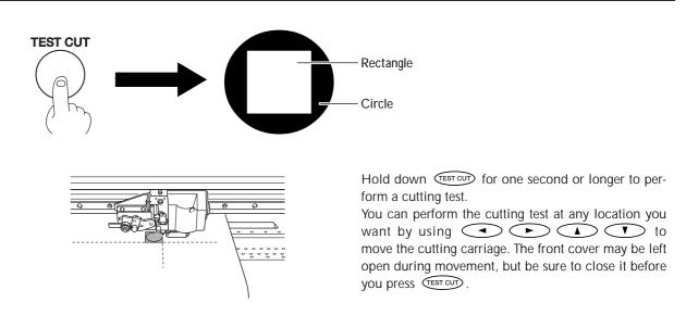
Peel off the cut shapes to verify the cutting quality, and make the setteing for blade force. For information on how to make the setting, refer to the next section.
