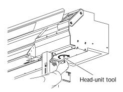
5. Make the guides at the edges of the print heads line up with the guides at the edges of the cap unit. Turn the tool further to bring the cap unit near the heads.
