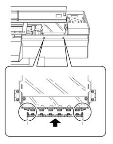
6. When the heads make contact with the cap unit, turn the tool one or two turns more.
