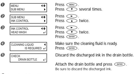
Thereafter, follow the on-screen instructions to carry out the operations. After cleaning has finished, the sub power is switched off.
