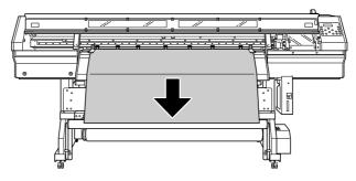
So Fasten the media in place with tape at three locations (the center and both edges) so that the media is not at an angle.
