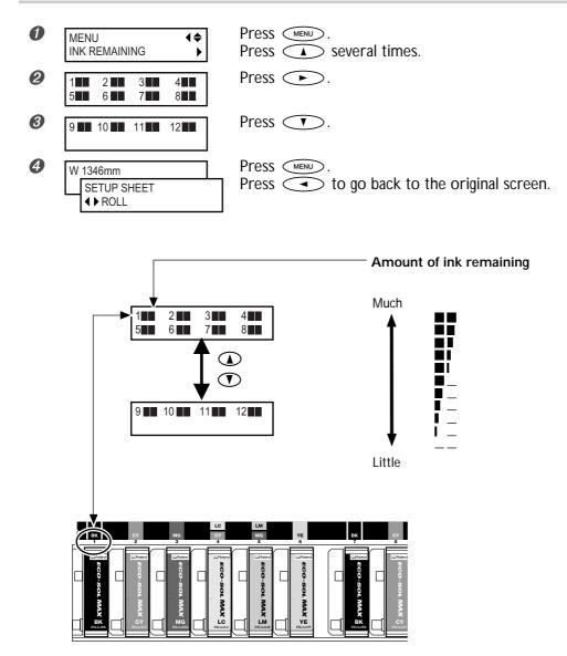
The display shows an approximate guide to the amount of remaining ink, which may differ somewhat from the actual amount remaining. Also, the displayed information may differ greatly from the actual amount remaining if you insert a partly used ink cartridge or change cartridges while the power is off.
