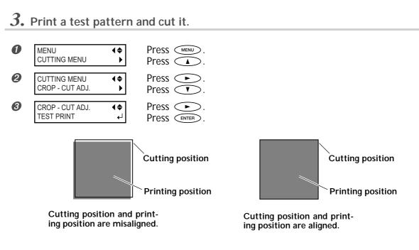
When adjustment is needed, go on to the steps below.
