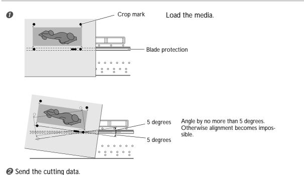
Alignment is performed automatically, then cutting starts.
