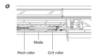
Pass the media between the pinch rollers and the grit rollers, bringing the end of the media as far as the platen.
