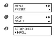
Use to select the name of a preset you want to load. Press to load. The settings are changed and the screen shown in the figure appears.
