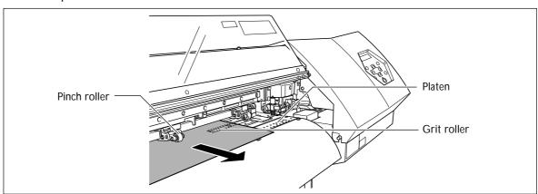
**6** Make sure both edges of the media are above the grit rollers, then place pinch rollers over all grit rollers covered by the media.
