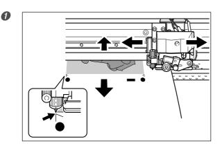
Use to align the center of the blade with the location shown in the figure.
