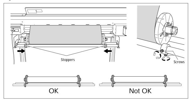
**6** Pass the leading edge of the media between the grit rollers and the pinch rollers, and feed it out as far as the platen.
