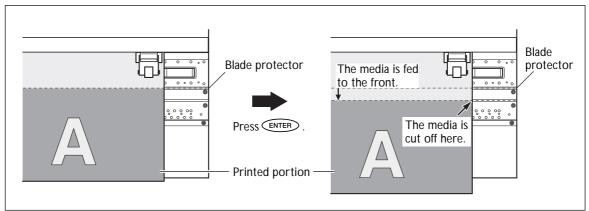
You can make the setting in the software RIP for automatic media cutoff after printing or cutting has finished. For information on how to make the setting, refer to the documentation for the software RIP you're using.
