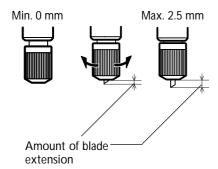
When you want to perform accurate and fine adjustment of the cutting-in amount, such as when cutting media with thin backing paper, you can obtain good results by adjusting the tip of the blade. Turn the cap portion of the blade holder to adjust the amount of blade extension. Each indicator tick corresponds to 0.1 millimeters, and adjustment for 0.5 millimeters can be made by rotating the cap one full turn.
