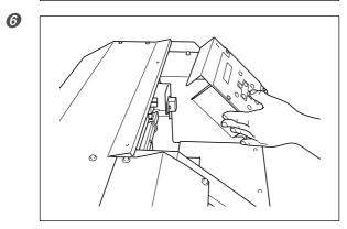
Touch the location shown in the figure to discharge any static electricity.
