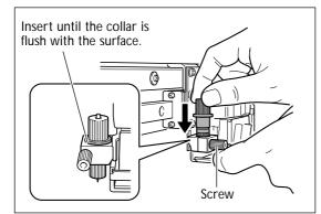
Support the screw from below and insert the blade holder.
