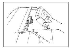
Touch the location shown in the figure to discharge any static electricity.
