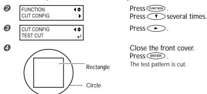
**5** Peel off the cut shapes to verify the cutting quality.
