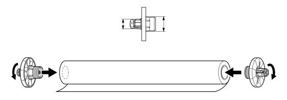
3 Place the roll media on the shafts and position its left and right edges to match the grit patterns.
