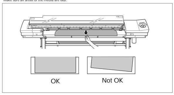
2 Lower the loading lever to hold the media in place.
