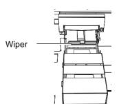
**5** Use a cleaning stick to wipe away any buildup of dust and grime from the wiper.
