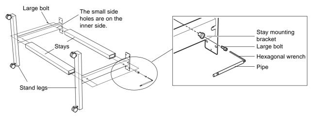
2 Set the stand upright and tighten the bolts securely.
