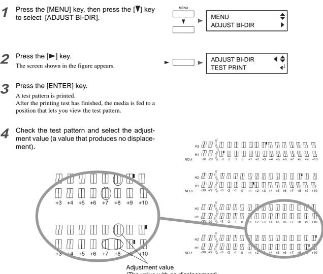
Adjustment value (The value with no displacement) In this figure, the No. 1 adjustment values are H1 = 7  $1/_2$  and H2 = 8.
