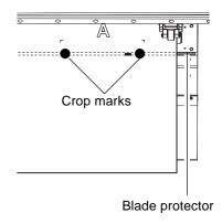
When you send data, alignment is performed automatically, then cutting starts.
