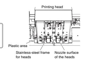
2 Clean the surface of the stainless-steel frame on the right side of the machine. Use a cleaning stick to wipe away any buildup of dust and ink from the surface of the stainless-steel frame.
