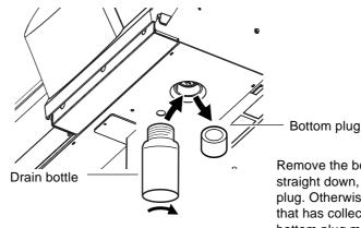
Remove the bottom plug by pulling straight down, without tilting the plug. Otherwise discharged fluid that has collected inside the bottom plug may spill.
