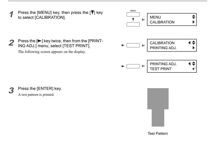
4 Check the printing result. If the correct result is not obtained, then proceed from step 5 and after. Refer to the figure below and modify the adjustment value.
