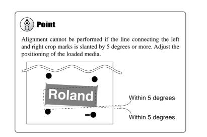
Align the crop marks with the blade protector and load a
