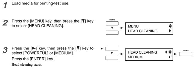
Men head cleaning finishes, perform a printing test to check the result.
